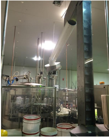
Capper conveyor. Pop top 5 head capper shown below:
