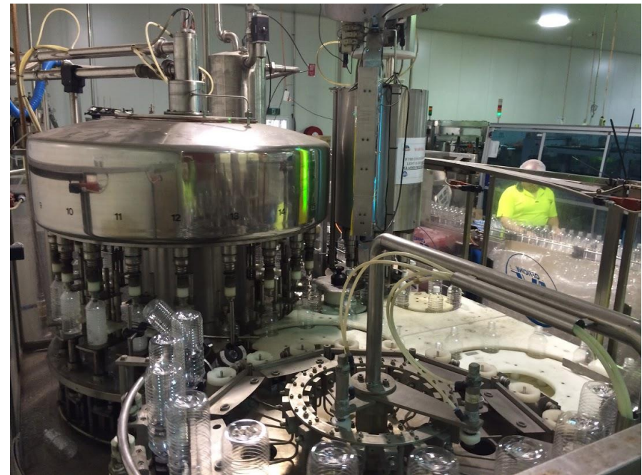
Change parts for 300ml, 350ml, 600ml, 750ml and 1500ml bottles.
